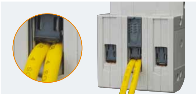
Terminals can accommodate 2 wires of same cross section (Solid up to 2 X 10 mm 2 and finely stranded with end sleeve up to 2 X 4 mm 2 ) without twisting wire strands facilitates easier and safe wiring
